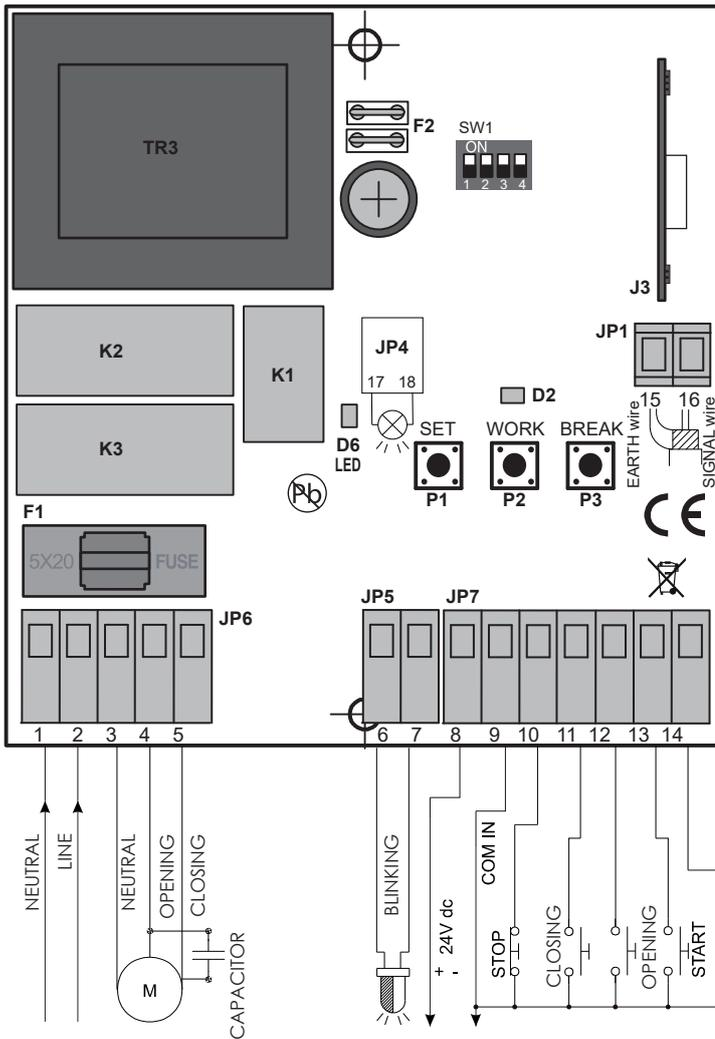
**Polarity in main power supply line connection must always be respected**
