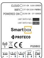
**V-in** Power input 12-24V DC, to be taken from the automation control board.
