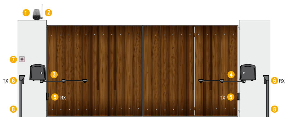
1_Flashing light 2_Standalone antenna 3_Control board 4_Key switch 5_Closing photocell 6_Opening photocell 7_Swing operators 8_Photocell posts
