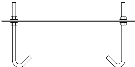
Picture 10: Anchor screws view
