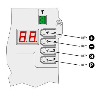
If you wish to reduce or increase the value of the setting use  $\bigcirc$   $\bigcirc$ . A **ttention!** when you reach the desired setting, wait shortly while the screen displayes the current value and setting alternatively. If you wish to move to a different setting, press  $\bigcirc$  and then  $\bigcirc$  as previously outlined.
