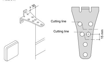
In order to properly cut the bracket start 15 mm from the hole center, as shown in the picture.
